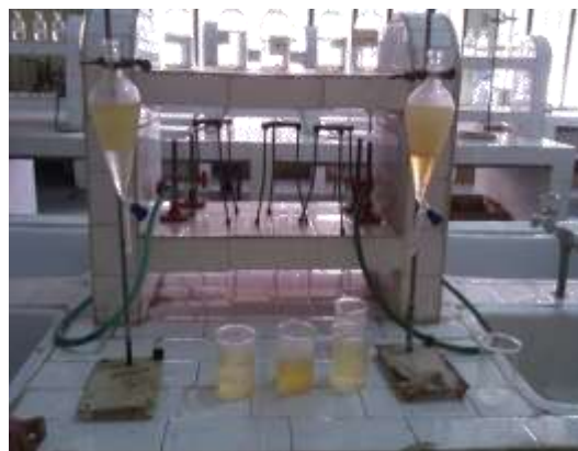
Figure 7: Water and Methyl Ester layers during separation
